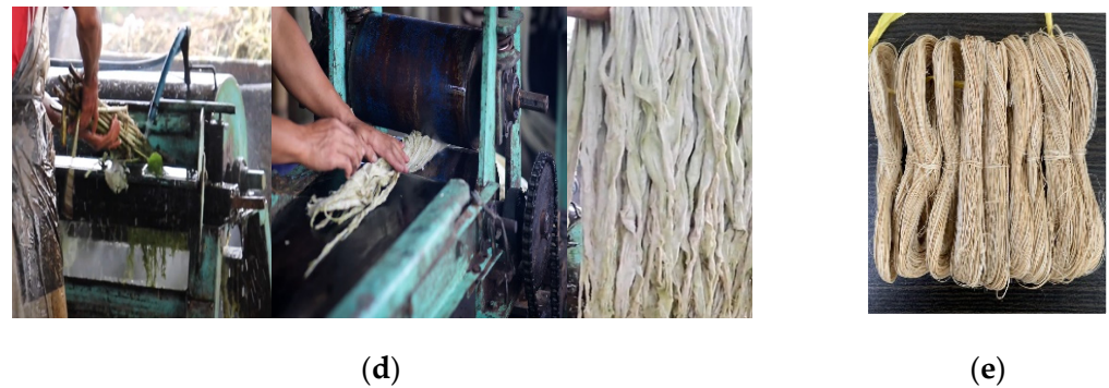
Figure 1. Process of ramie fiber yarn extraction: (a) Ramie. (b) Harvesting. (c) Steaming of ramie. (d) Ramie yarn fiber decorticated. (e) Extracted ramie yarn fiber.
