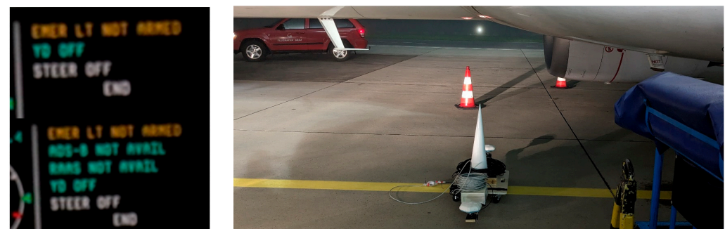
Figure 4. (Left): Display of ADS-B and RAAS availability in cockpit. If jamming with enough power, “ADS-B NOT AVAIL” and “RAAS NOT AVAIL” are displayed in green color, as can be seen from the lower panel (no better picture quality possible). (Right): “Center” position of jammer below the aircraft.
