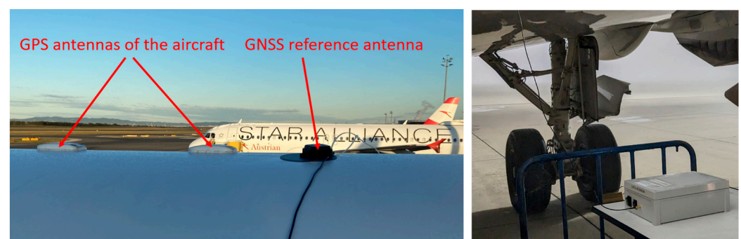
Figure 2. (Left): Positioning of GNSS reference antenna on top of aircraft. (Right): Sensor box below aircraft, placed on a table and connected via cable to GNSS reference antenna.
