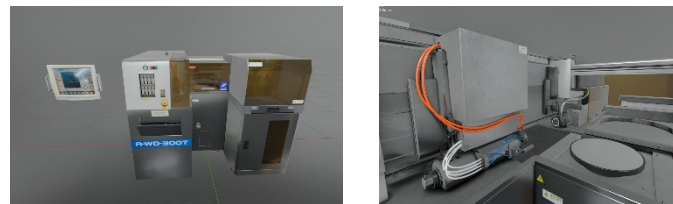
Figure 3. The picture on the left is a 3D digital simulation of a wafer-slicing machine. The picture on the right is a digital twin close-up of the process of replacing the cutting blade.
