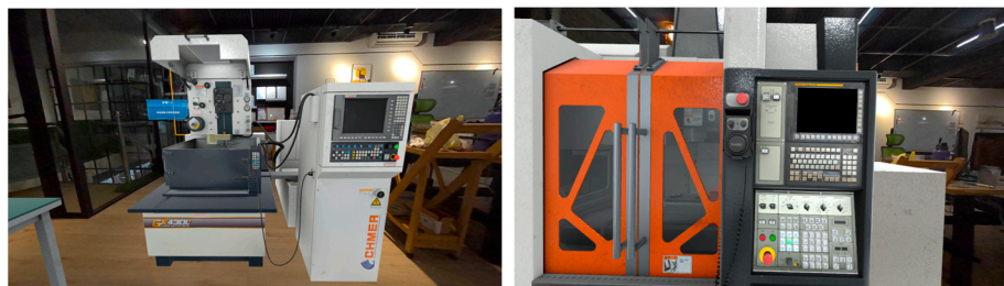
Figure 1. Concept of DT: The picture on the left is the digital twin of the wire cutting machine. The picture on the right is a digital twin of a six-axis machining center.
