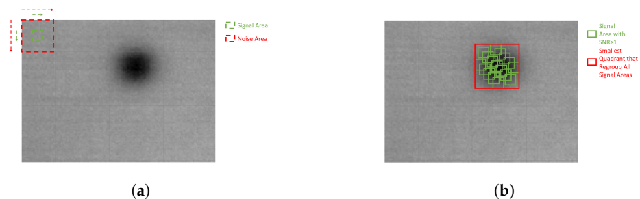
Figure 3. Automatic defect detection. (a) Selection of noise and signal areas. (b) Defect detection.
