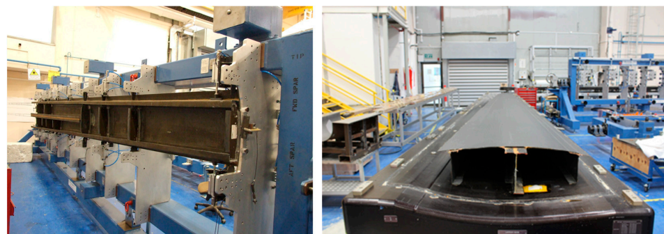
Figure 2. Composite full-scale manufactured wing box.
