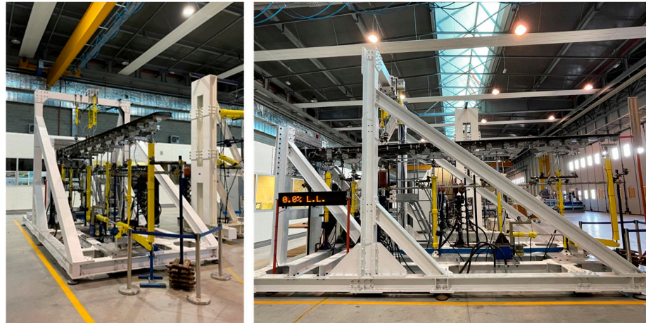
Figure 4. Full-scale composite wing box installed on test rig @ Piaggio Aerospace Lab.
