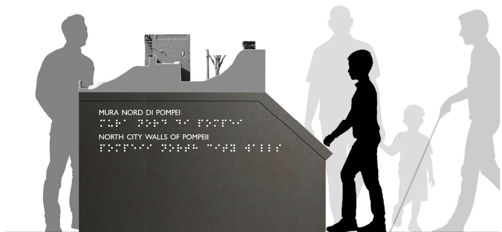
Figure 8. Design of the museum installation displaying the 1:1-scale 3D-printed prototypes of wall cavities and stone balls, with reference to the significant wall section, allowing tactile interaction.
