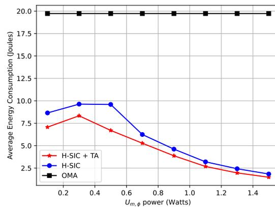
Figure 6. Average energy consumption versus  $U_{m,\phi}$ 's power.
