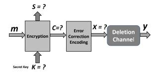
Figure 2. Model of encryption for cryptanalysis at the attacker's side under known plaintext attack.
