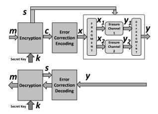
Figure 1. Security enhanced encryption scheme.
