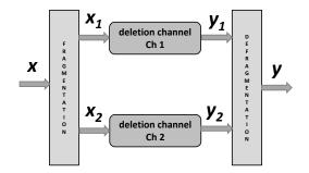
Figure 3. Model of the deletion channel with frangmentation.
