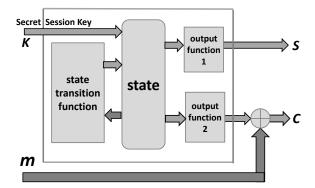
Figure 4. Model of encryption based on a stream cipher.
