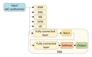
**Figure 10.** The AC coefficients as input for the multilayer fully connected neural network and the classifiers.
