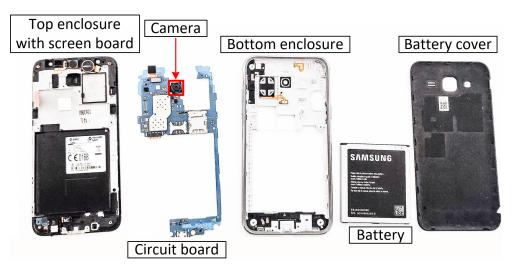
Figure 4. Samsung Galaxy J5 dismantled to replace the camera.
