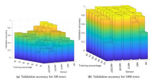
**Figure 15.** Validation accuracy for 2, 3, 4, 5, and 6 sensors for 100 randomly selected rows (**a**) and 1000 randomly selected rows (**b**) in the case of the WNN classifier.
