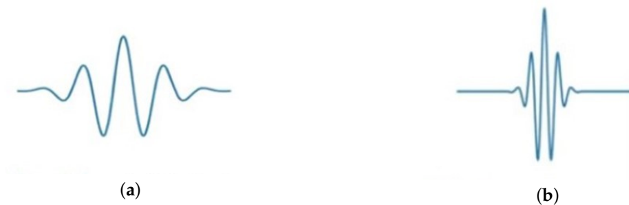
Figure 5. (a) Expanded wavelet for resolving low-frequency components. (b) Shrunk wavelet for resolving high-frequency components.
