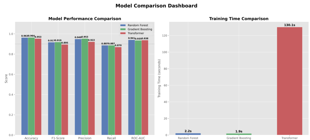
Figure 5. Overall performance and training-time comparison of Random Forest, Gradient Boosting, and the proposed transformer-based model.
