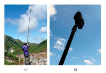
**Figure 4.** (**a**) A 4-m long pole with a camera held by an operator; (**b**) Camera mounted at the end of the pole (Photos: T. Wang, 6 September 2017).
