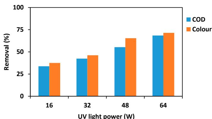
**Figure 4.** Effect of UV light irradiation power on photocatalytic degradation (process conditions: pH—4, reaction time—3 h,  $\text{TiO}_2$  dosage—500 mg/L).
