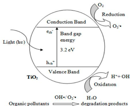
**Figure 1.** Photocatalytic mechanism for  $\text{TiO}_2$  photocatalyst.
