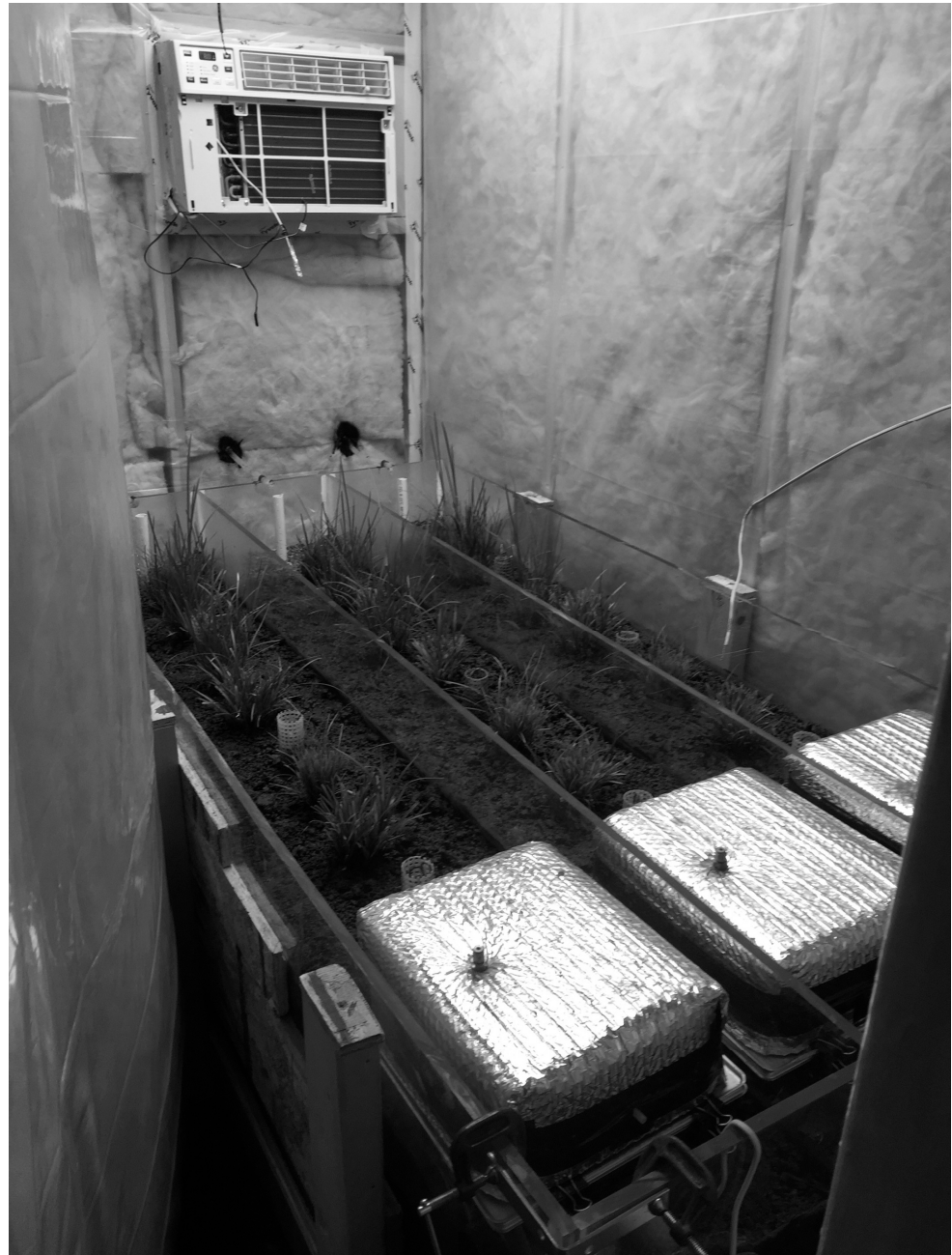
Figure 1. Photo of experimental bioreactors inside a temperature control chamber (2.44 m × 1.22 m × 1.83 m) as part of the testing apparatus.
