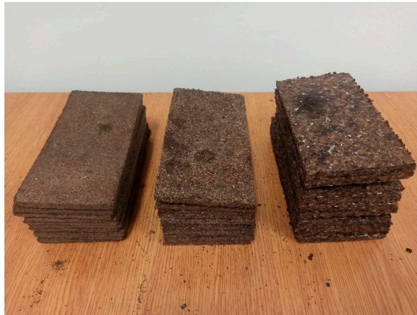
Figure 1. Buckwheat husk boards prepared from size fractions below 1 mm (left), 1–2 mm (middle), and raw (right).
