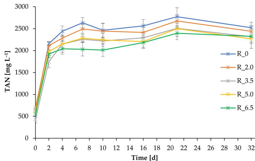
**Figure 5.** Impact of CNT addition on TAN accumulation during the anaerobic digestion of chicken manure. Different concentrations of CNTs ( $2.0 \text{ g L}^{-1}$ ,  $3.5 \text{ g L}^{-1}$ ,  $5.0 \text{ g L}^{-1}$ , and  $6.5 \text{ g L}^{-1}$ ) were added to the reactors (R\_2.0, R\_3.5, R\_5.0, and R\_6.5, respectively). R\_0 operated without the addition of CNTs.
