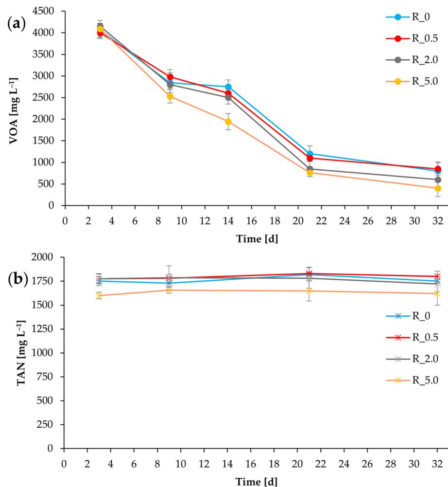
**Figure 2.** Impact of CNT addition on VOA concentrations (a) and TAN concentrations (b) during the anaerobic digestion of chicken manure. Different concentrations of CNTs (0.5 g L<sup>-1</sup>, 2.0 g L<sup>-1</sup>, and 5.0 g L<sup>-1</sup>) were added to the reactors (R\_0.5, R\_2.0, and R\_5.0, respectively). R\_0 operated without the addition of CNTs.
