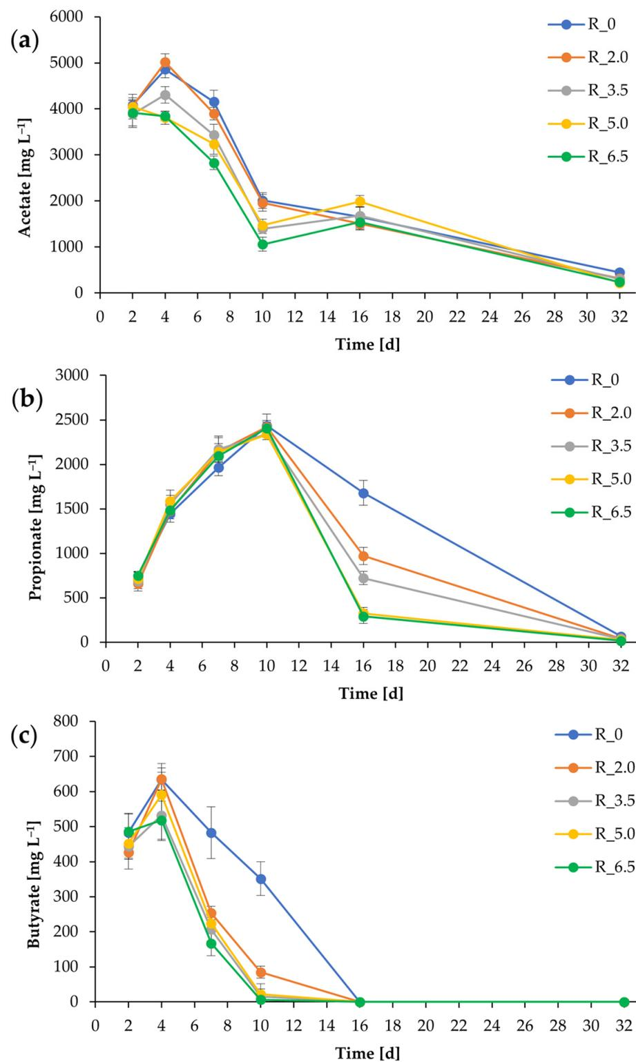
**Figure 4.** Impact of CNT addition on acetate (a), propionate (b), and butyrate (c) during the anaerobic digestion of chicken manure. Different concentrations of CNTs (2.0 g L<sup>-1</sup>, 3.5 g L<sup>-1</sup>, 5.0 g L<sup>-1</sup>, and 6.5 g L<sup>-1</sup>) were added to the reactors (R\_2.0, R\_3.5, R\_5.0, and R\_6.5, respectively). R\_0 operated without the addition of CNTs.
