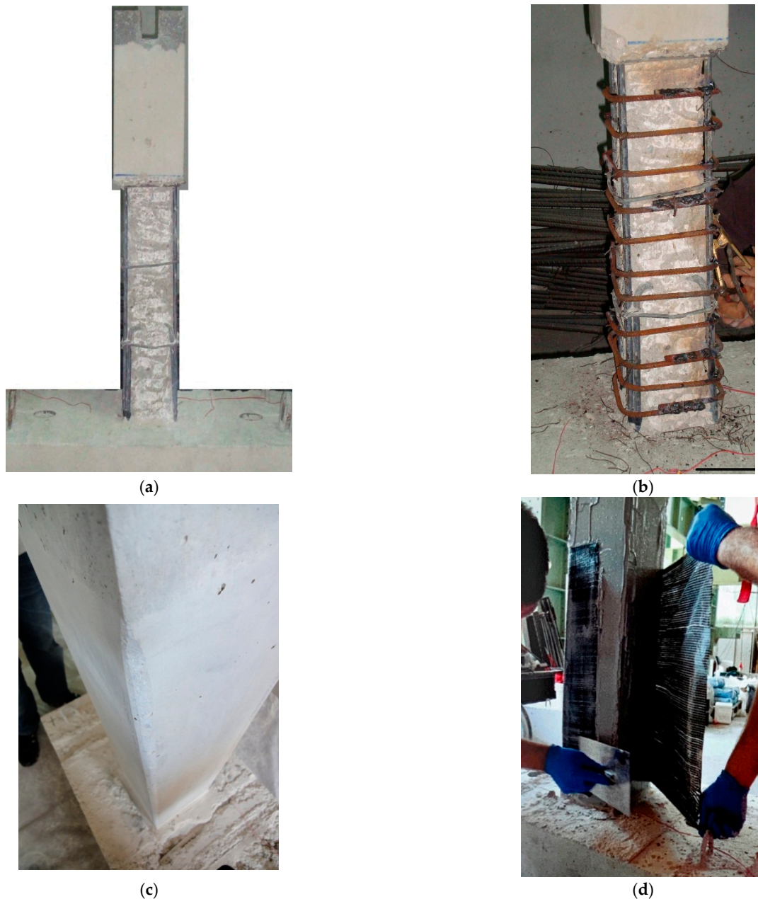
Figure 2. Strengthening interventions (a) specimens RG 1 and RG 2 : the concrete cover is chipped-away; (b) specimens RG 1 and RG 2 : the ties of the thin high-strength RC jacket are placed in touch with the initial column; (c) specimen FS 2 : smoothing of the column surface and curving of the column edges; (d) specimen FS 2 : wrapping of the CFRP textile and full integration to the resin matrix.
