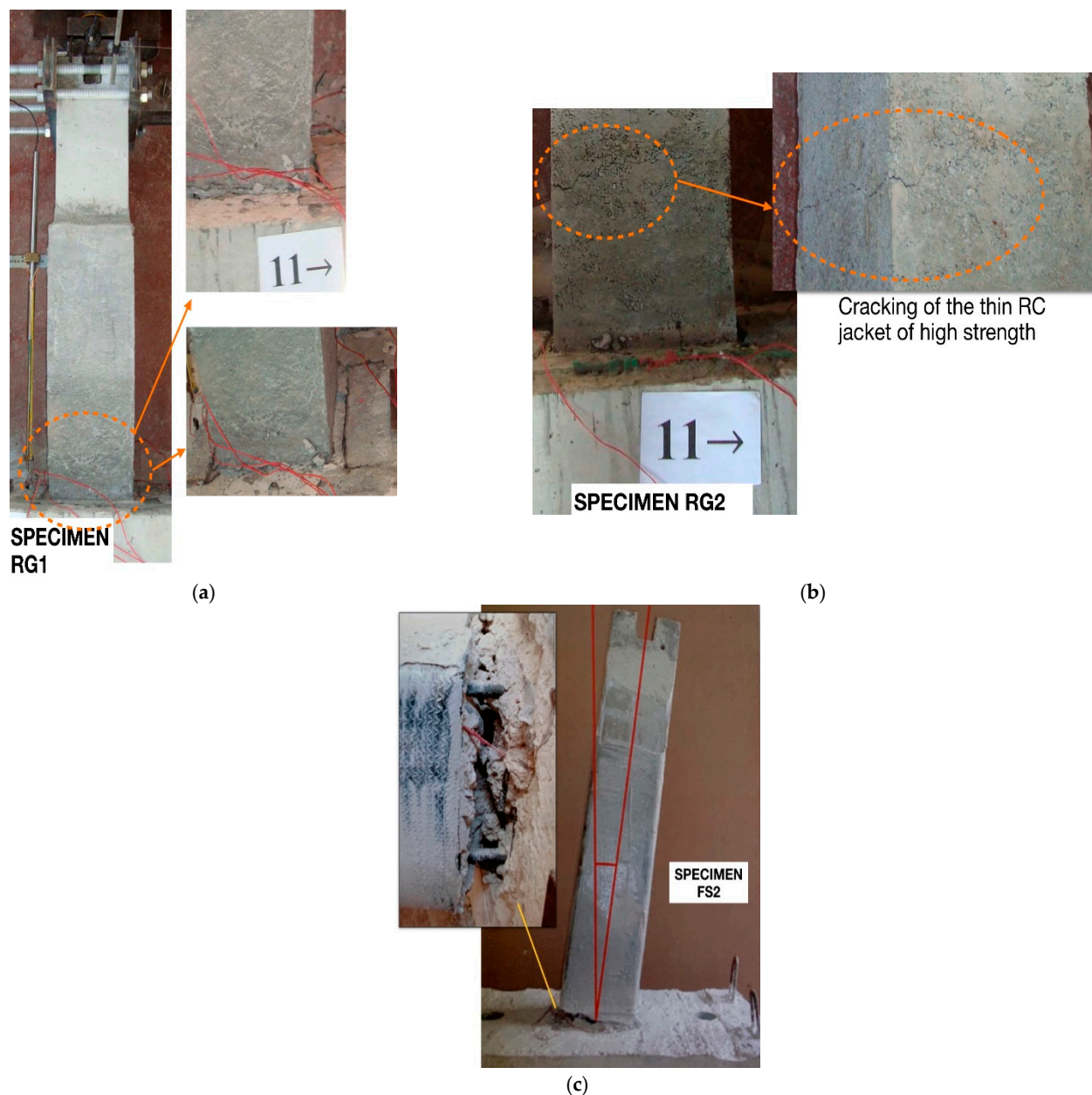
Figure 8. Failure modes of column specimens (a) RG 1 and (b) RG 2 strengthened with thin high-strength RC jacket and (c) of specimen FS 2 strengthened with CFRP jacket of two layers of textile.
