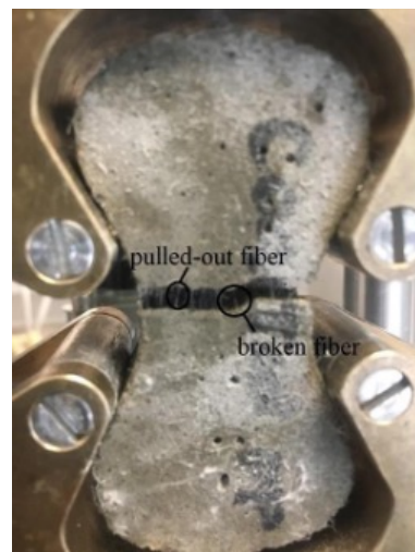
Figure 9. Coated PP-reinforced mortar under tension.
