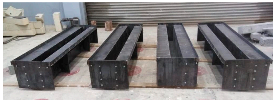
(a) Steel mold formwork
