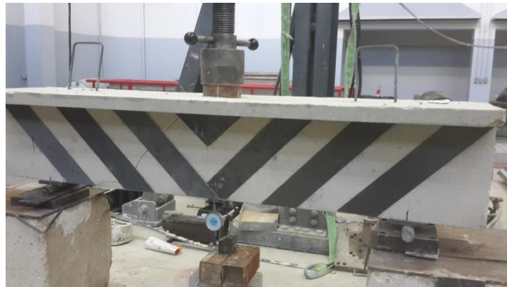
(a) Group 2 shear failure
