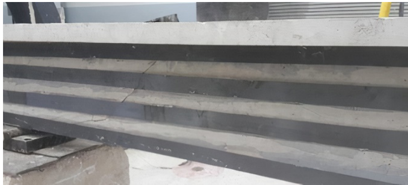
(c) Group 3 shear failure
