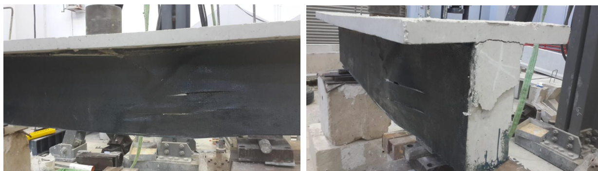
(e) Group 4 failure mode
