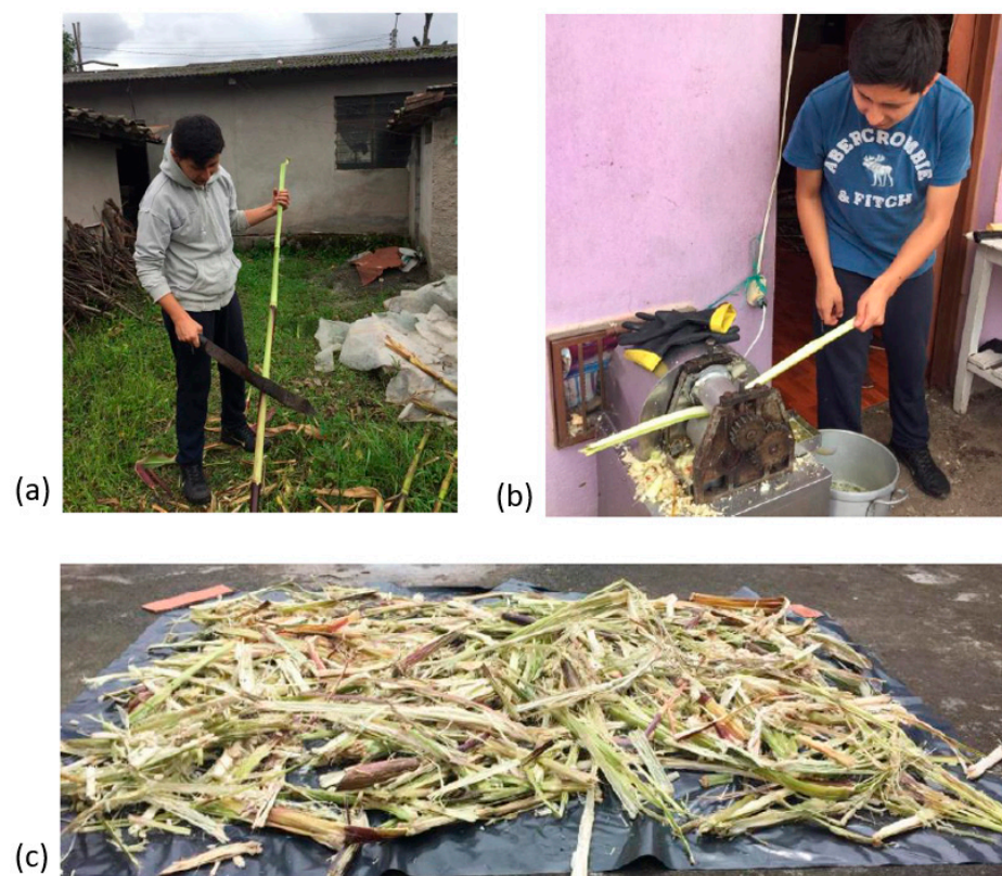
Figure 2. (a) Process of separating unnecessary parts of the plant; (b) crushing in a machine to extract juice from the stem; (c) drying the crushed fiber exposed to the weather for a period of two days (48 h).
