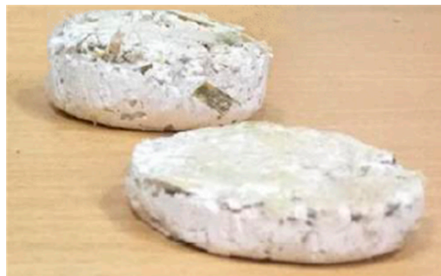
Figure 3. Samples for measurement in the impedance tube.
