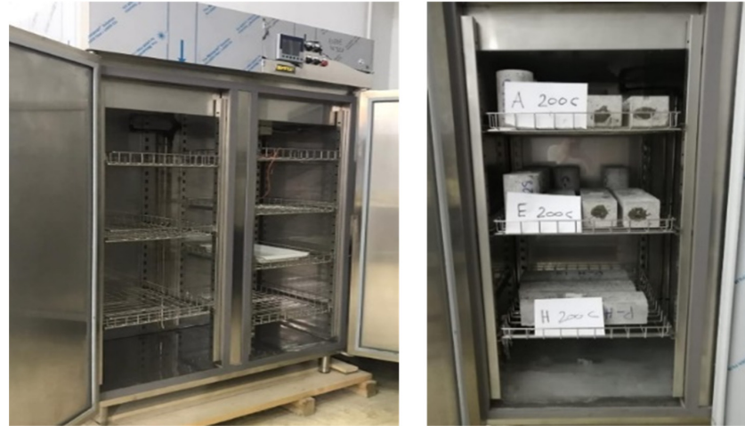
Figure 6. Specimens before being subjected to freeze-thaw cycles.
