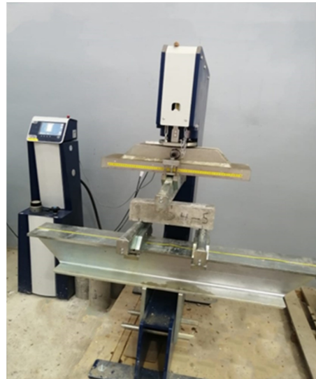
Figure 5. Flexural test of SCC specimens.
