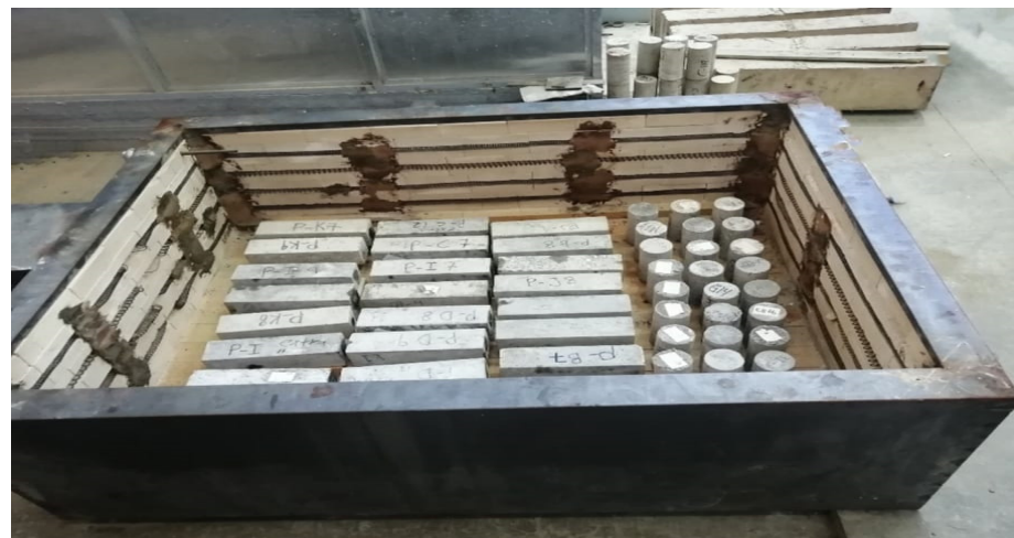
Figure 7. The samples before being subject to high temperatures in a furnace.
