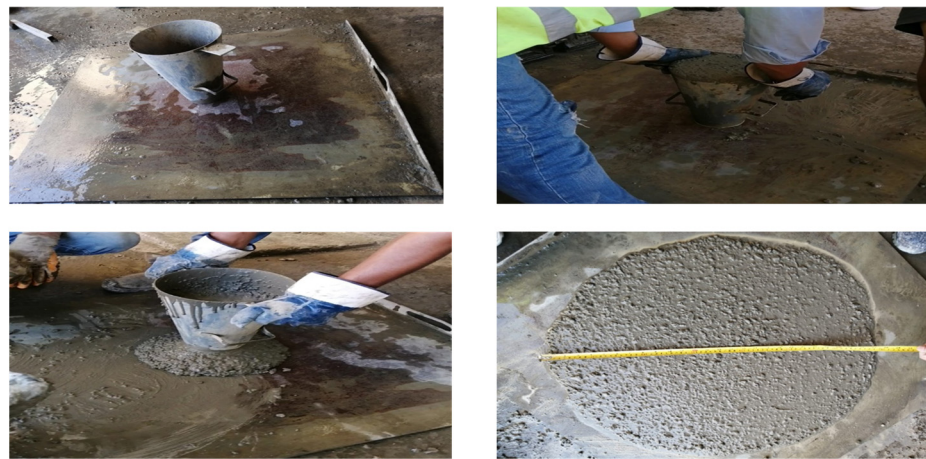
Figure 3. Steps of the slump flow test.
