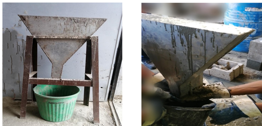
Figure 4. Steps of the V-funnel test.
