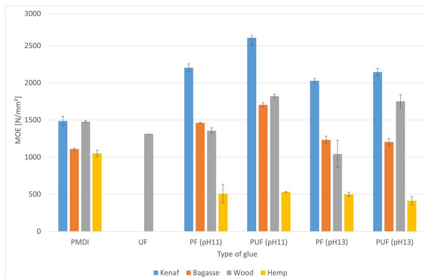
Figure 6. MOE for the biocomposites made from the four fibers.
