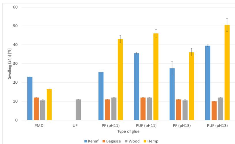
Figure 8. TS 24 h for the biocomposites made from the four fibers.
