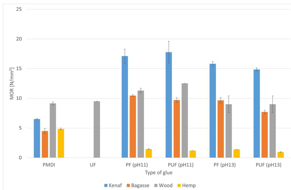
**Figure 5.** MOR for the biocomposites made from the four fibers.
