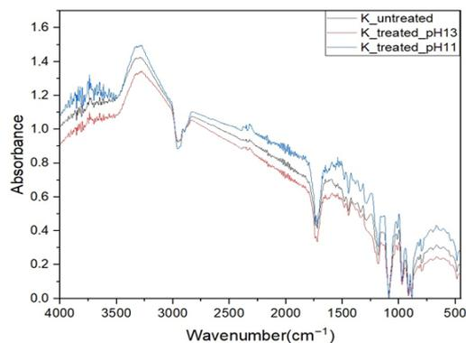
Figure 2. Fourier transform infrared spectroscopy analysis (FTIR) of untreated and treated Kenaf fiber at pH 11 and pH 13.
