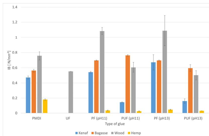
**Figure 4.** Internal bond for the biocomposites made from the four fibers.
