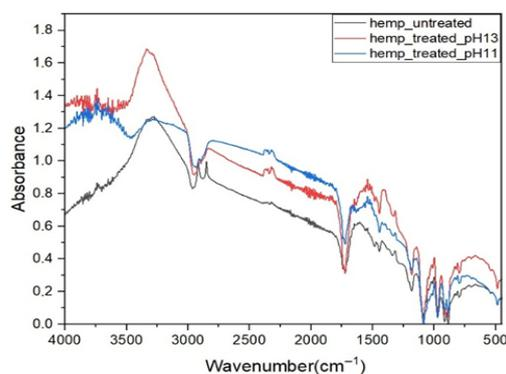
Figure 3. Fourier transform infrared spectroscopy analysis (FTIR) of untreated and treated Hemp fiber at pH 11 and pH 13.
