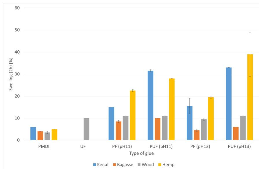
Figure 7. TS 2 h for the biocomposites made from the four fibers.
