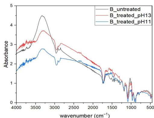
**Figure 1.** Fourier transform infrared spectroscopy analysis (FTIR) of untreated and treated Bagasse fiber at pH 11 and pH 13.
