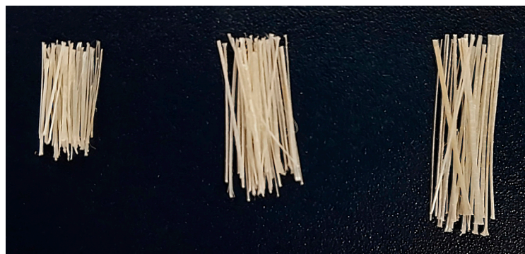
Figure 3. Abacá fibers with lengths of 5 mm, 10 mm, and 15 mm were used.
