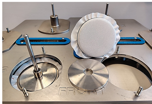
Figure 1. Induction of surface pilling on viscose fabric specimens by rubbing against standard wool abrasant fabric using the Martindale pilling tester 2561 E, Mesdan S.p.A., Raffa, Italy.
