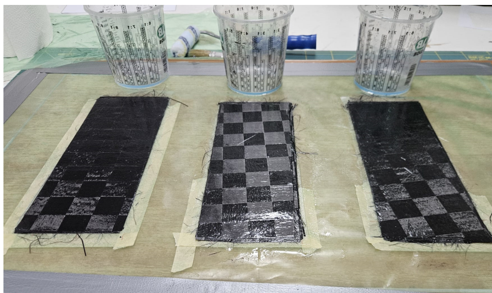
Figure 2. Plates during hand lay-up process.
