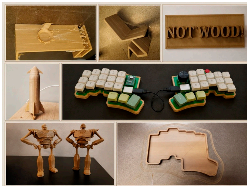
Figure 10. Representative print operational validation objects produced using 30SHF/PLA bio-composite filament (only the left humanoid figure in the bottom left image was printed using 10SHF filament).
