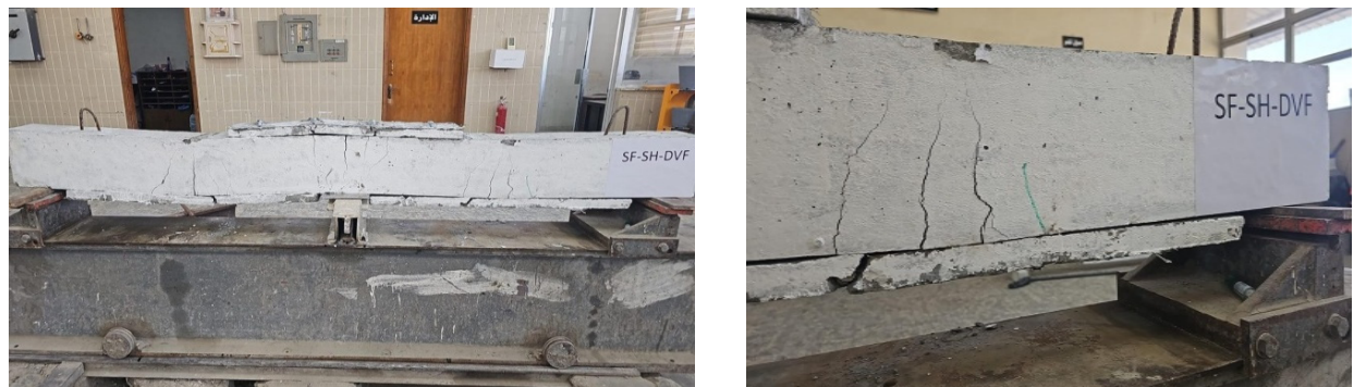
Figure 13. Failure mode and crack propagation of the SF-SH-DVF beam.
