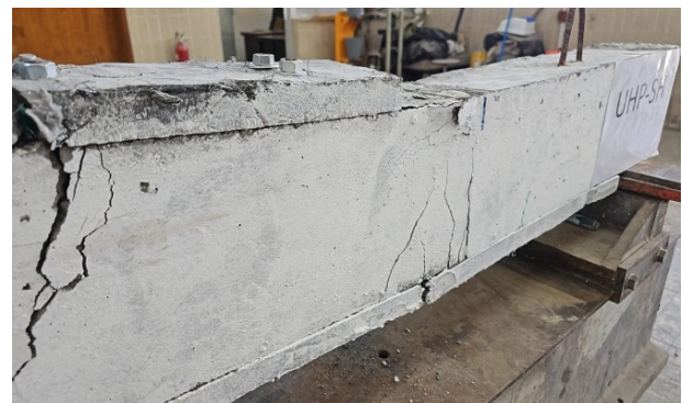
Figure 17. Failure mode and crack propagation of the UHP-SH beam.
