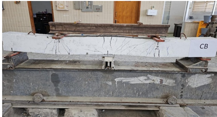
Figure 9. Failure mode and crack propagation of the control beam.
