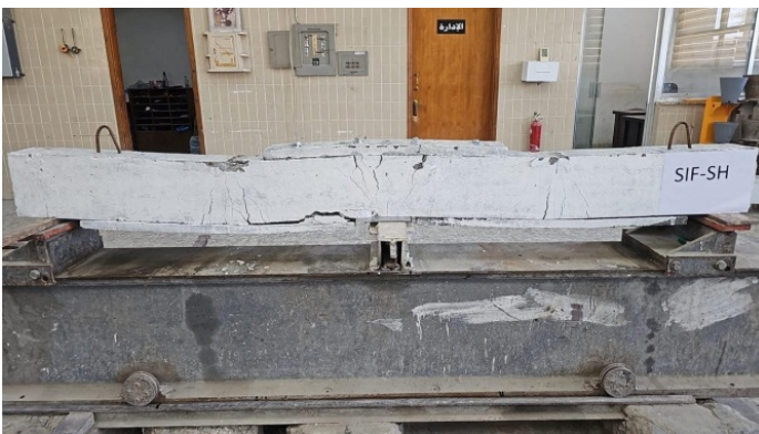
Figure 18. Failure mode and crack propagation of the SIF-SH beam.
