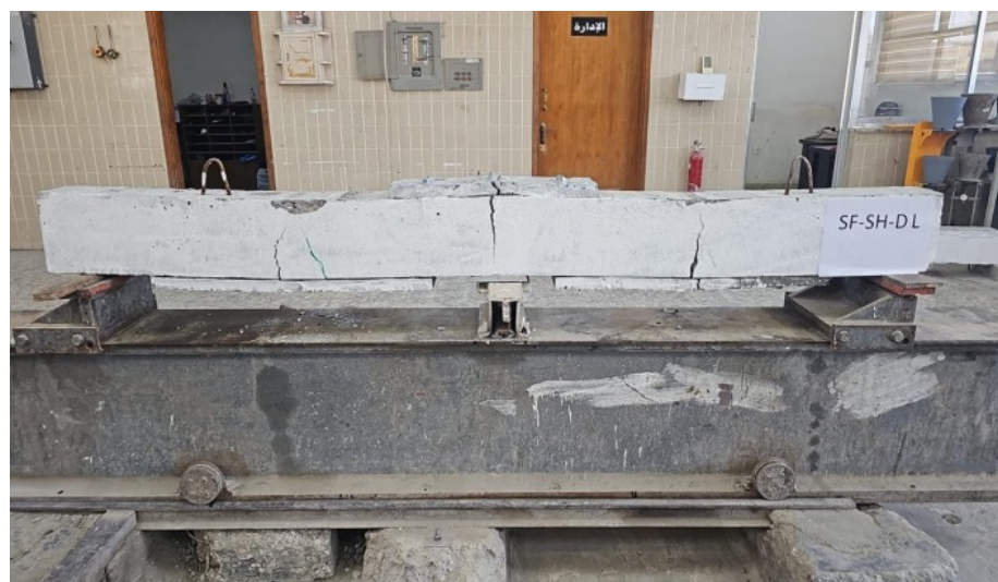
Figure 11. Failure mode and crack propagation of the SF-DL beam.
