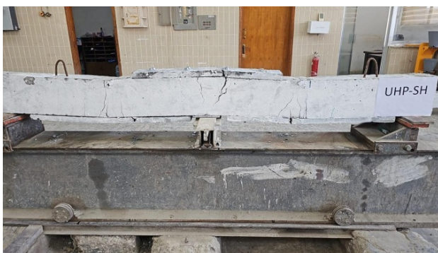
Figure 17. Failure mode and crack propagation of the UHP-SH beam.
