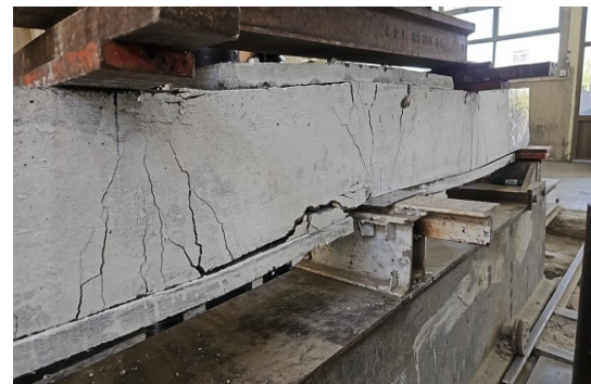
Figure 18. Failure mode and crack propagation of the SIF-SH beam.
