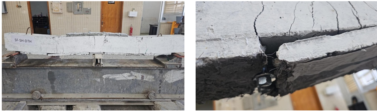
Figure 12. Failure mode and crack propagation of the SF-SH-DTH beam.
