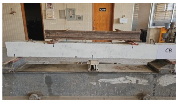
(a) Four point load test
