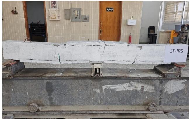
Figure 16. Failure mode and crack propagation of the SF-IRS beam.
