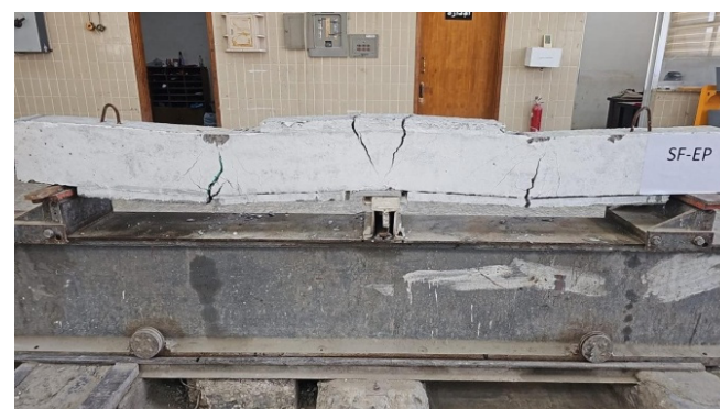
Figure 15. Failure mode and crack propagation of the SF-EP beam.
