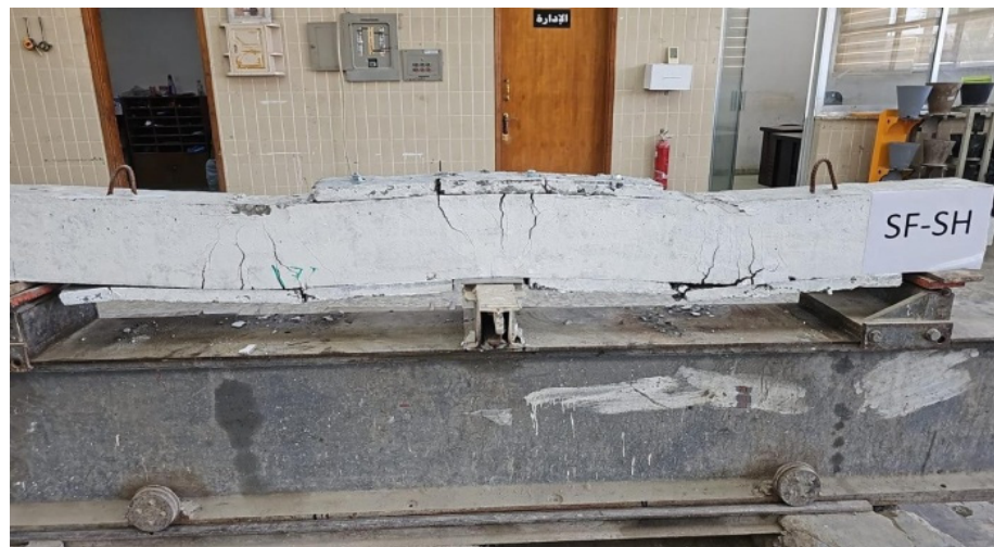
Figure 10. Failure mode and crack propagation of the SF-SH beam.
