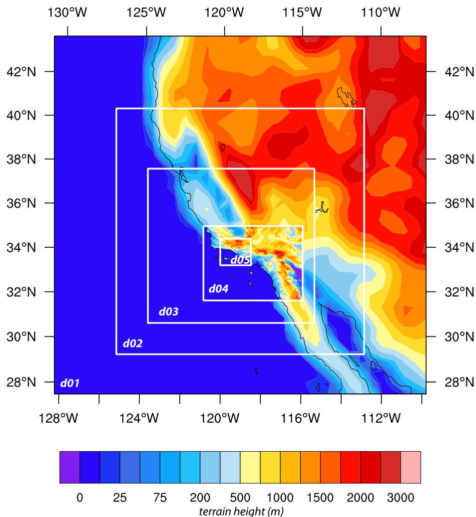
**Figure 3.** Telescoping configuration employed for most of the WRF simulations in this study (see Table 1), consisting of five (54, 18, 6, 2, and 0.667 km horizontal grid spacing) domains and based on [6,15], except that the innermost nest was shifted over the Thomas Fire area. Topography of outermost domain shown (shaded), except where superimposed with 2 km (Domain 4) terrain. Verifications against observations discussed herein were performed in Domain 4.
