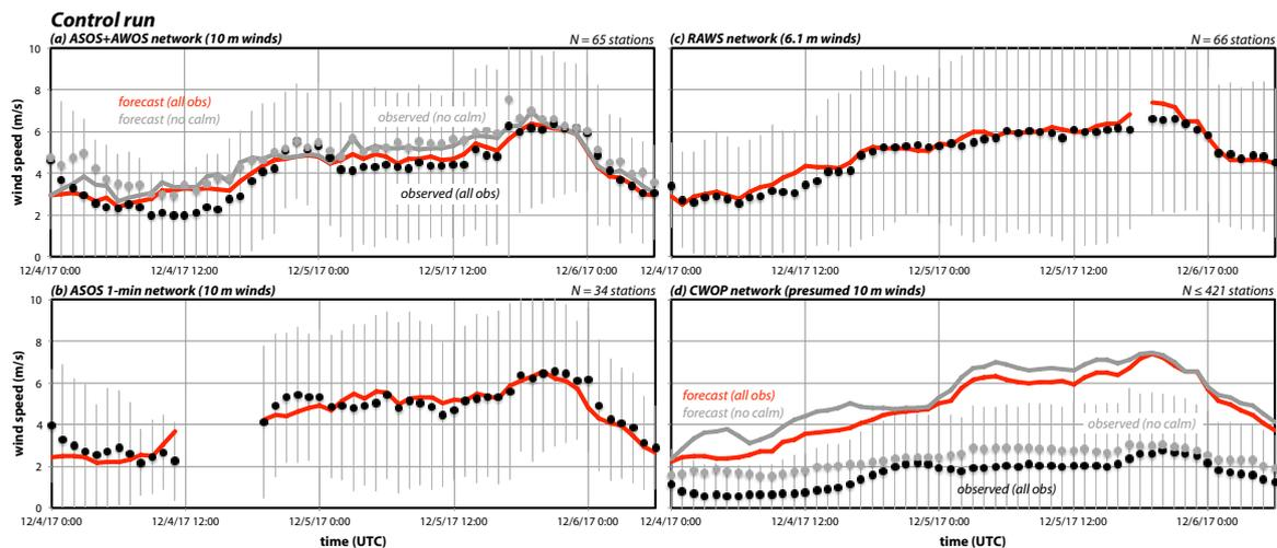
**Figure 8.** Network-averaged sustained wind observations (black dots) and forecasts (red curves) for (a) ASOS + AWOS, (b) ASOS 1-min, (c) RAW5, and (d) CWOP over the simulation period. Vertical grey lines denote  $\pm 1$  standard deviation around the observations. In (a,d), network averages disregarding calm observations and corresponding forecasts are represented as grey dots and lines, respectively; for (c) one forecast hour was neglected owing to observation dropouts.
