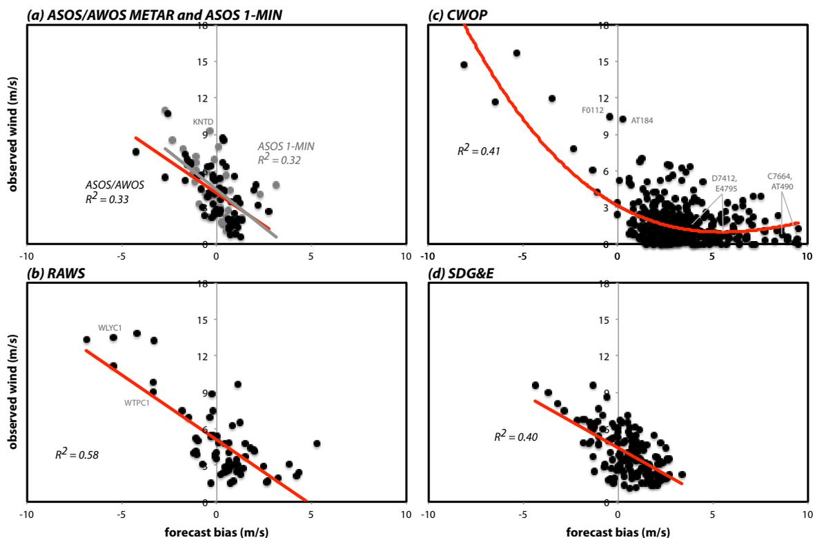
**Figure 10.** Station-average sustained wind forecast bias vs. observed sustained wind speed (black or grey dots) along with least squares fits (red lines) for the (a) ASOS+AWOS and ASOS 1-min, (b) RAWS, (c) CWOP, and (d) SDG & E networks. Regressions are shown to emphasize correlations but are not used in this analysis.
