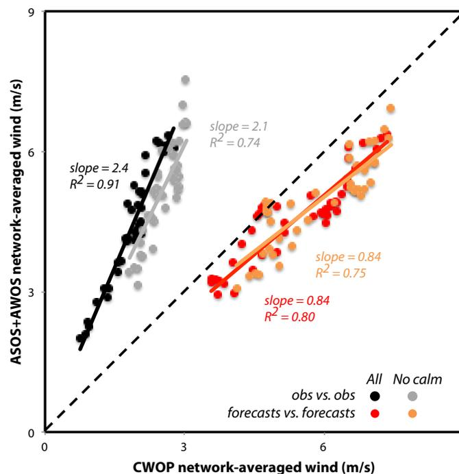
**Figure 9.** Comparison of network-averaged CWOP (horizontal axis) vs. ASOS + AWOS (vertical axis) observations (black dots) and corresponding forecasts (red dots), hourly between forecast hours 12–54, inclusive. Observation (grey dots) and forecast (orange dots) comparisons after calm and/or low quality observations were removed are also shown. The linear fits are depicted as solid lines corresponding to their subset's colors. The black dashed line represents one-to-one correspondence.
