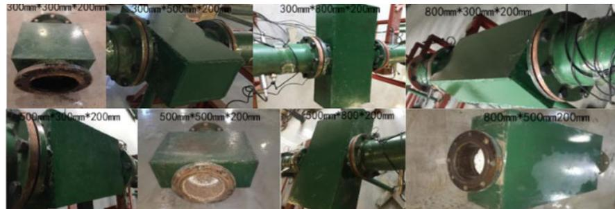
**Figure 3.** Physical model of the explosion chamber.
