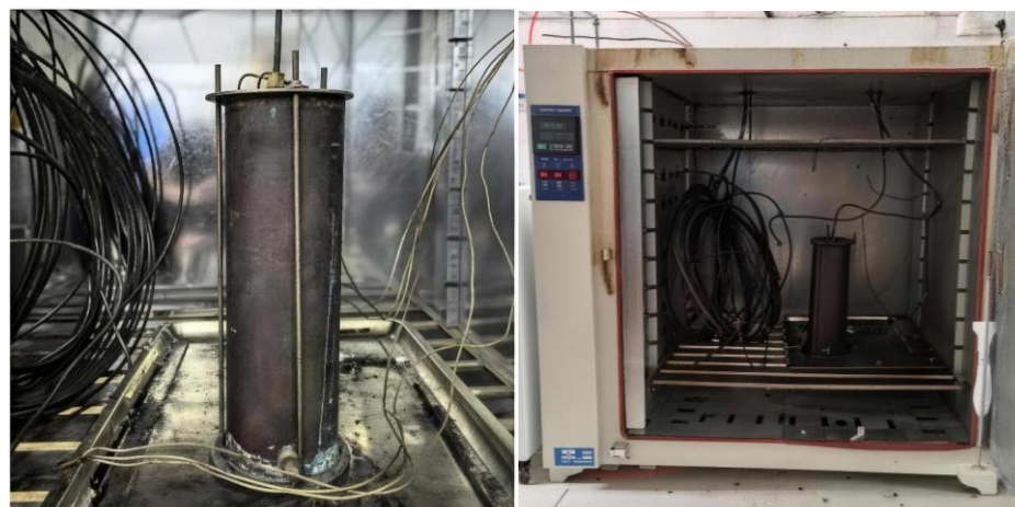
Figure 2. Photographs of the coal reaction vessel and electrothermal blast drying oven.
