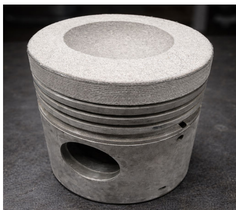
Figure 5. Plasma-sprayed ceramic-coated piston crown.
