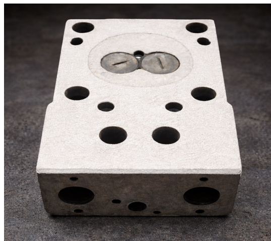
Figure 4. Plasma-sprayed ceramic-coated cylinder head.
