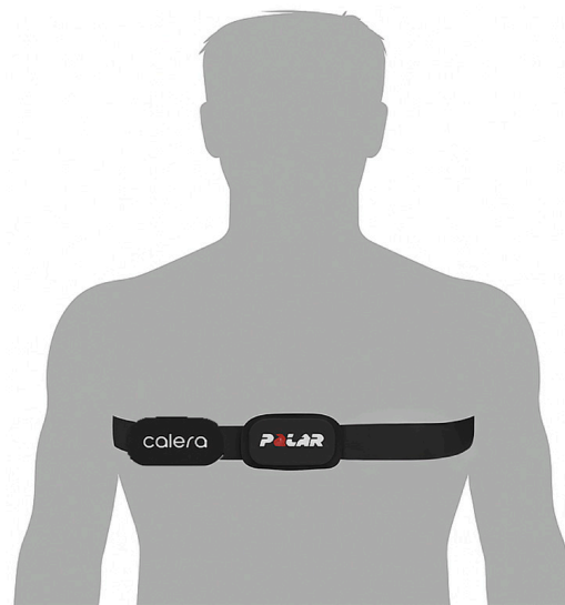
Figure 2. The heart rate monitor was placed in the center of the chest at the sternum, and the temperature sensor was placed to the right of the heart rate monitor on an elastic strap.
