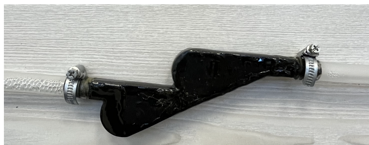
Figure 3. 3D-printed Tesla valve.
