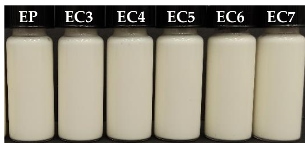
Figure 1. Visual appearance of cream-type emulsions (24 h after production). EP—cream-type emulsions based on palm oil; EC3/4/5/6/7—cream-type emulsions based on oleogel with 3, 4, 5, 6, or 7% w/w candelilla wax.
