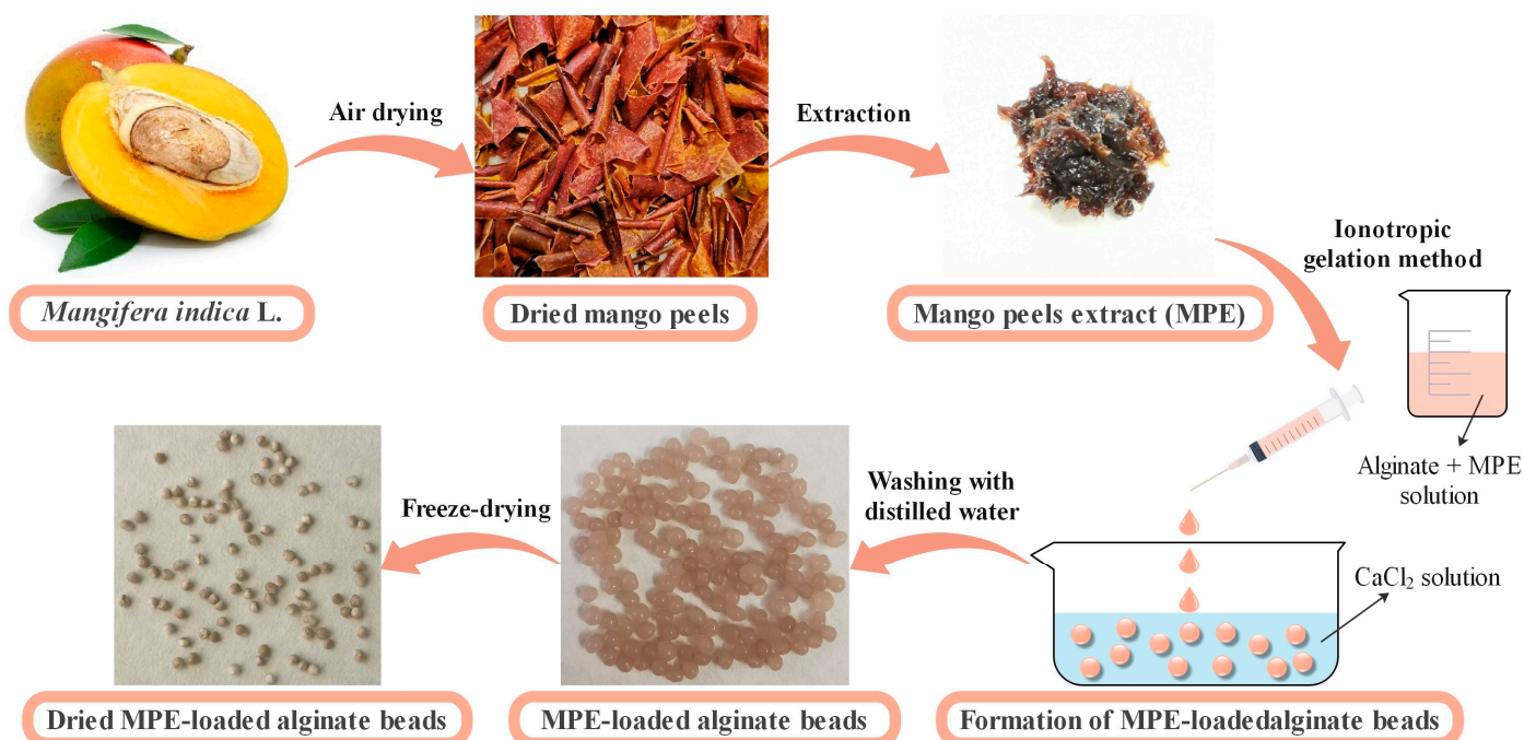
Figure 1. Schematic representation of MPE-loaded alginate bead preparation by ionotropic gelation method.
