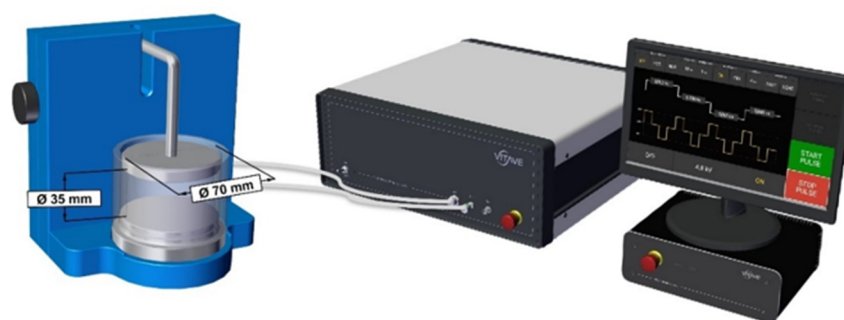
Figure 1. OmniPEF LAB generator with touch-display and high-voltage generator (r.) linked to a batch-treatment chamber (l.) (The exemplary illustration was provided by Vitave Tech, Prague, Czech Republic and was slightly adapted).
