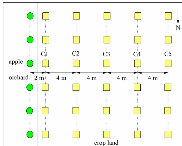
**Figure 2.** The layout of the soil moisture monitoring sites.
