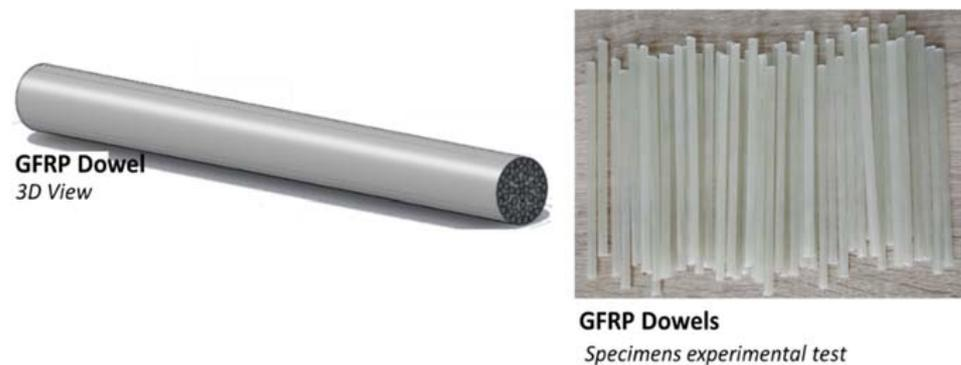
**Figure 3.** GFRP dowel specimens.
