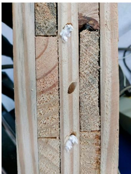
**Figure 9.** GFRP dowel failure mode for butt-end connections.
