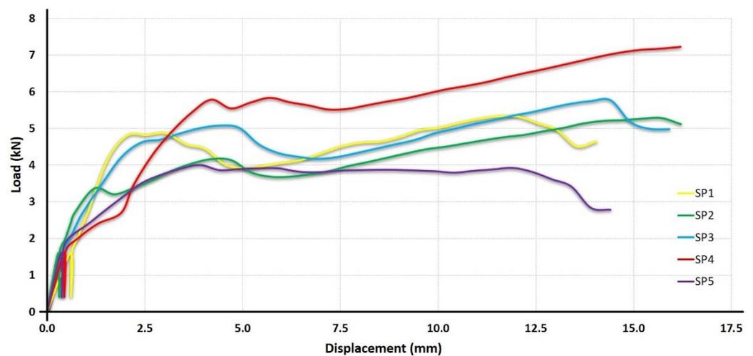
Figure 5. Load x displacement curves of butt-end connections (T1).
