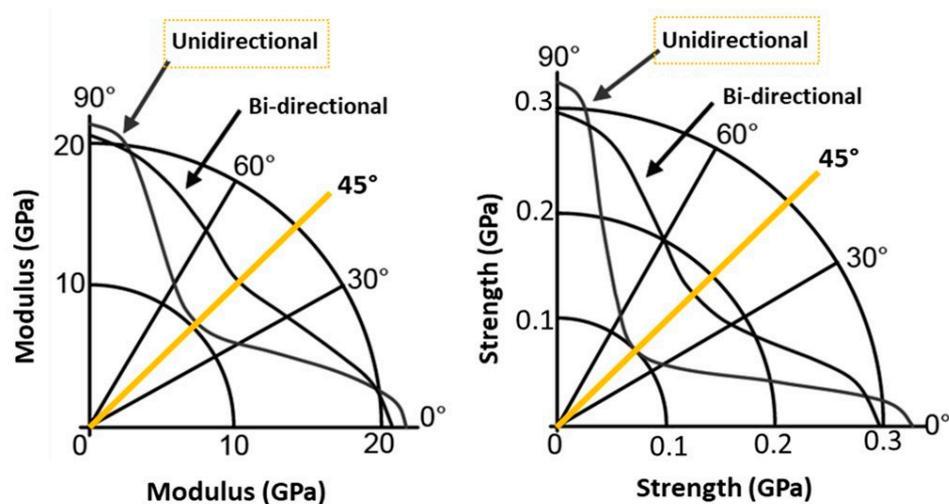
**Figure 8.** GFRP modulus of elasticity (MOE) and modulus of rupture (MOR) diagram as a function of the fiber orientation; source: Piggot [22].
