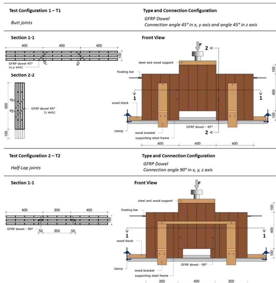
**Figure 2.** Test setups of configurations T1 and T2 (measures in mm).
