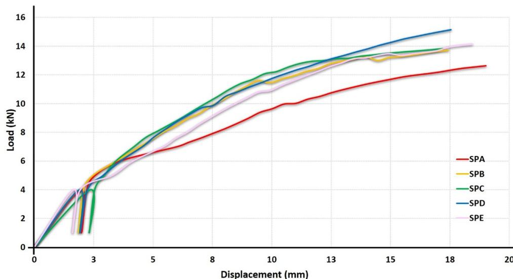
Figure 6. Load–displacement curves from half-lap connections (T2).
