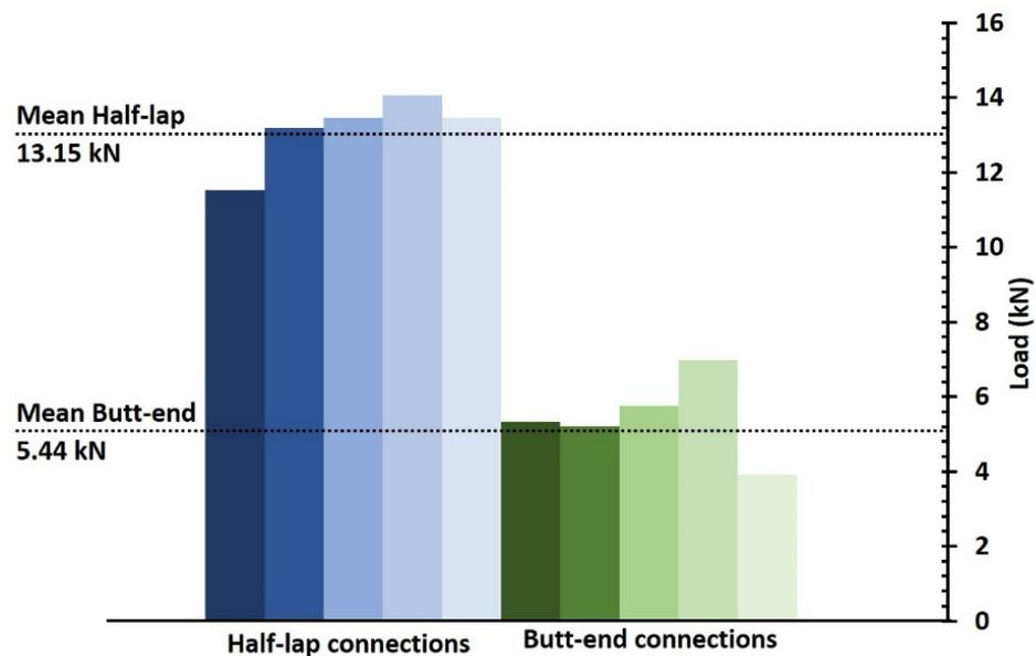
**Figure 7.** Comparison of mean maximum load ( $F_{max}$ ) of butt-end and half-lap connections.
