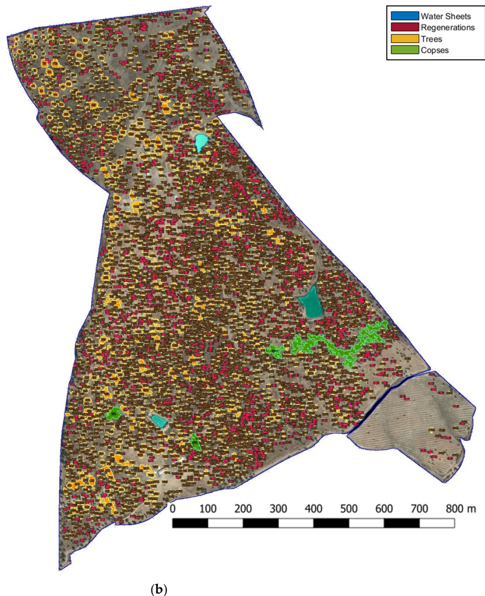
Figure 14. (a) Images input; (b) the images processed by the tools. Dark pink for regenerates, yellow for individual trees, green for copses and blue for water sheets.
