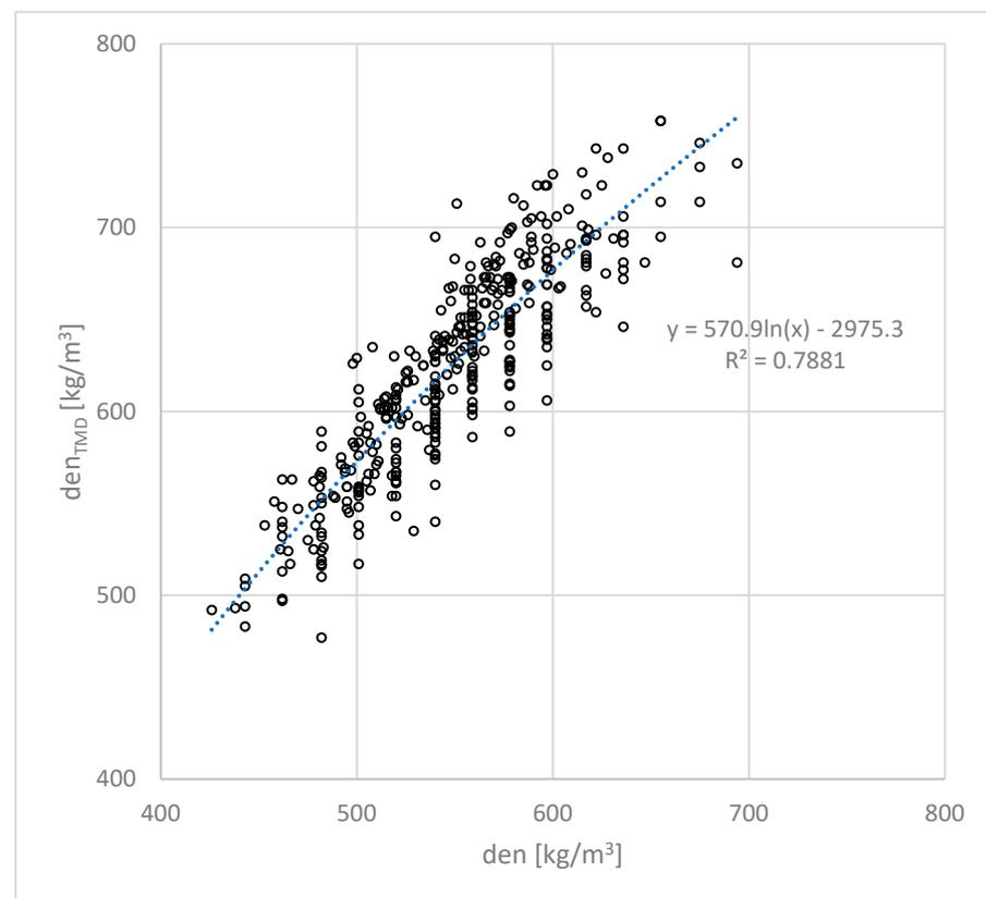
**Figure 1.** Relation between timber density before and after densification.
