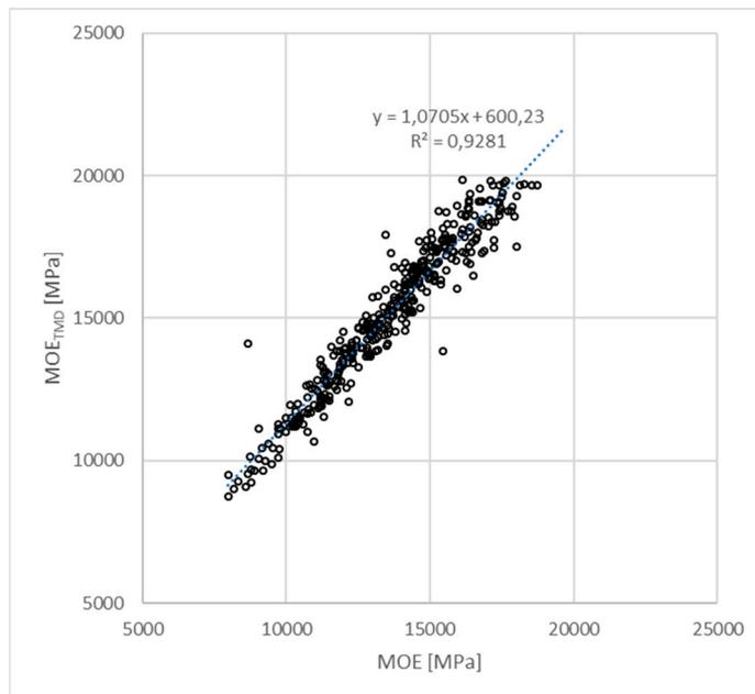
**Figure 5.** Relation between MOE before and after densification.
