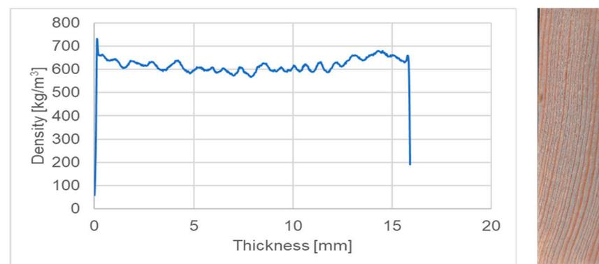
**Figure 4.** Density profile and cross-section of sawn timber after thermo-mechanical densification, average density of sample 615 kg/m<sup>3</sup>. Sawn timber after densification was planed on both sides to achieve flatness.
