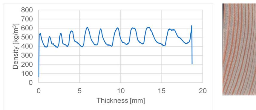
**Figure 3.** Density profile and cross-section of sawn timber before thermo-mechanical densification, average density of sample 482kg/m<sup>3</sup>. Sawn timber samples before modification were planed on both sides to achieve flatness.
