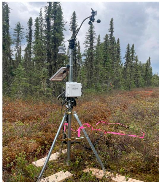
**Figure 2.** The meteorologic station set up on the EW seismic line. The tower includes an anemometer, relative humidity and temperature sensor, soil moisture and soil temperature sensors, and a tipping bucket rain gauge.
