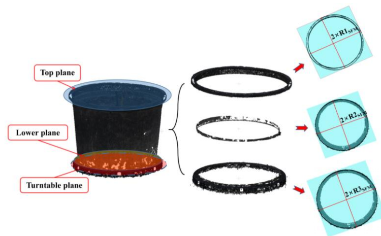
Figure 5. Point cloud shape and size calibration.
