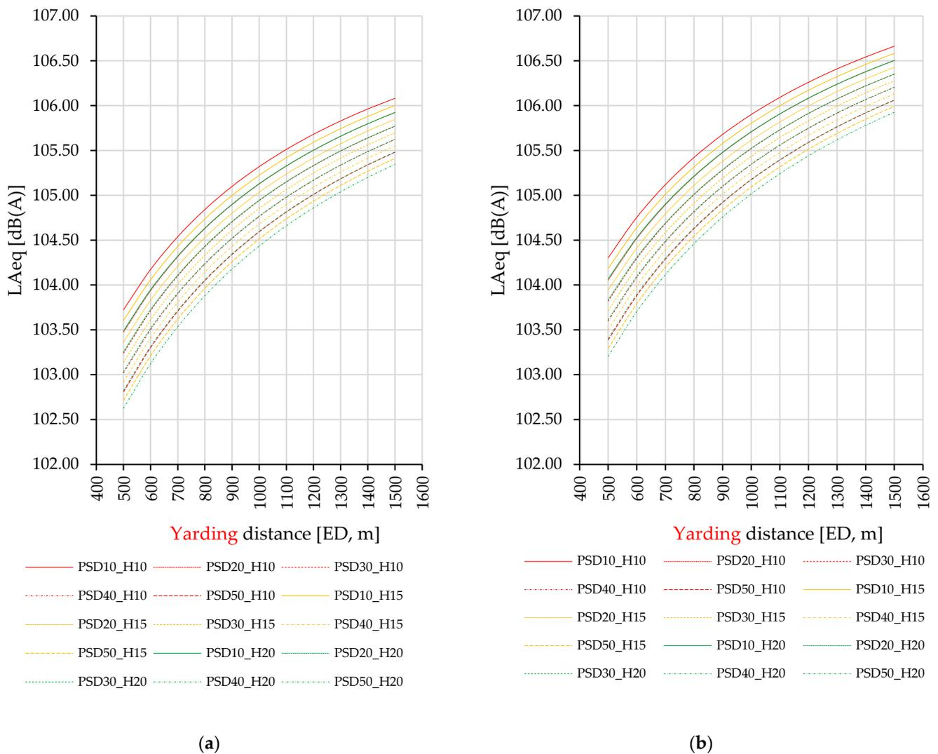
**Figure 4.** Exposure to noise depending on yarding distance (ED, m), lateral yarding distance (PSD, m), and skyline height (H): (a) simulated exposure to noise based on data considering a 1-h break during the day; (b) simulated exposure to noise based on data calculated for 7 h of work.
