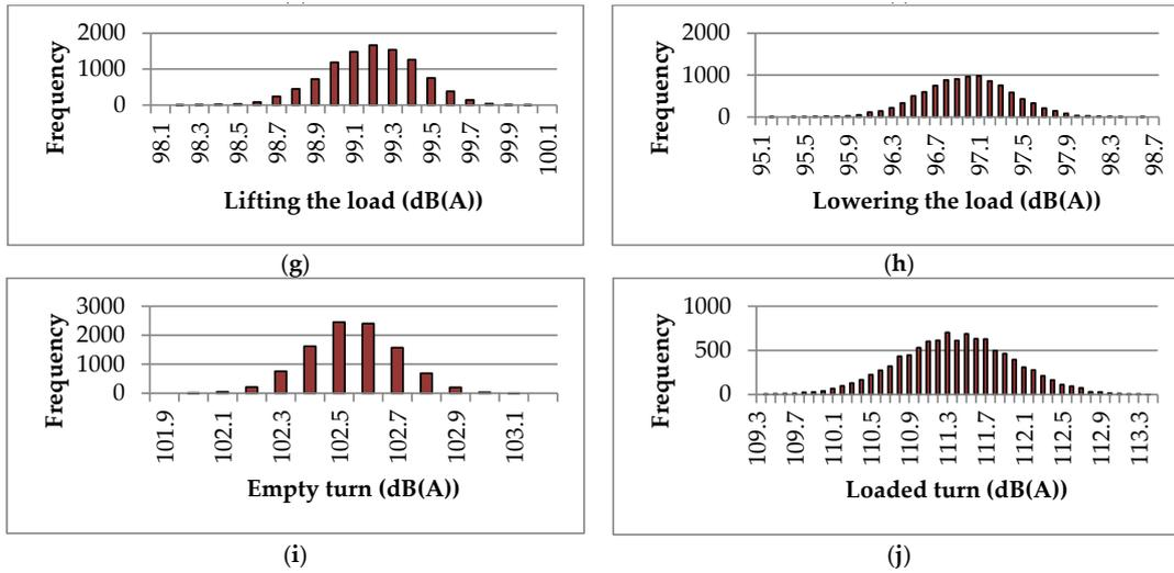
**Figure A1.** Frequency histograms of the parametric bootstrapping: (a) Engine off, (b) Engine off, cooling, (c) Engine on, no work, (d) Cable work, (e) Lifting the cable, (f) Lowering the cable, (g) Lifting the load, (h) Lowering the load, (i) Empty turn, (j) Loaded turn.
