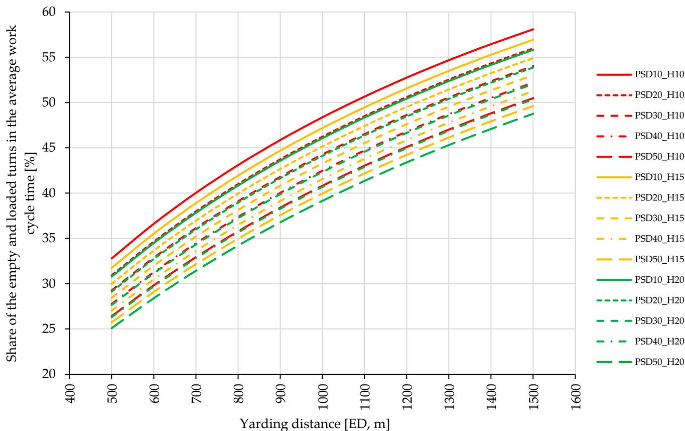
**Figure 3.** Share of empty and loaded turn times in the average work cycle time, depending on yarding distance (ED), lateral yarding distance (PSD), and skyline height (H). Note: PSD10 to PSD50—lateral yarding distances of 10 to 50 m, H10 to H20—skyline heights of 10 to 20 m.
