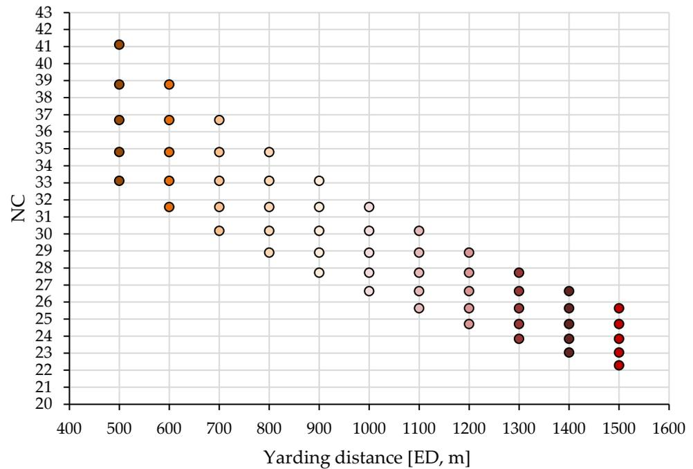
**Figure A2.** An example of the number of work cycles (NC) by considering a fixed skyline height (H) of 10 m, a variation in yarding distance (ED) from 500 to 1500 m, and a variation in lateral yarding distance (PSD) from 10 to 50 m. Note: for each yarding distance, from top to bottom, the number of work cycles that can be covered in 7 h of effective work, when increasing the lateral yarding distance from 10 (top) to 50 m (bottom), with a step of 10 m, is shown.
