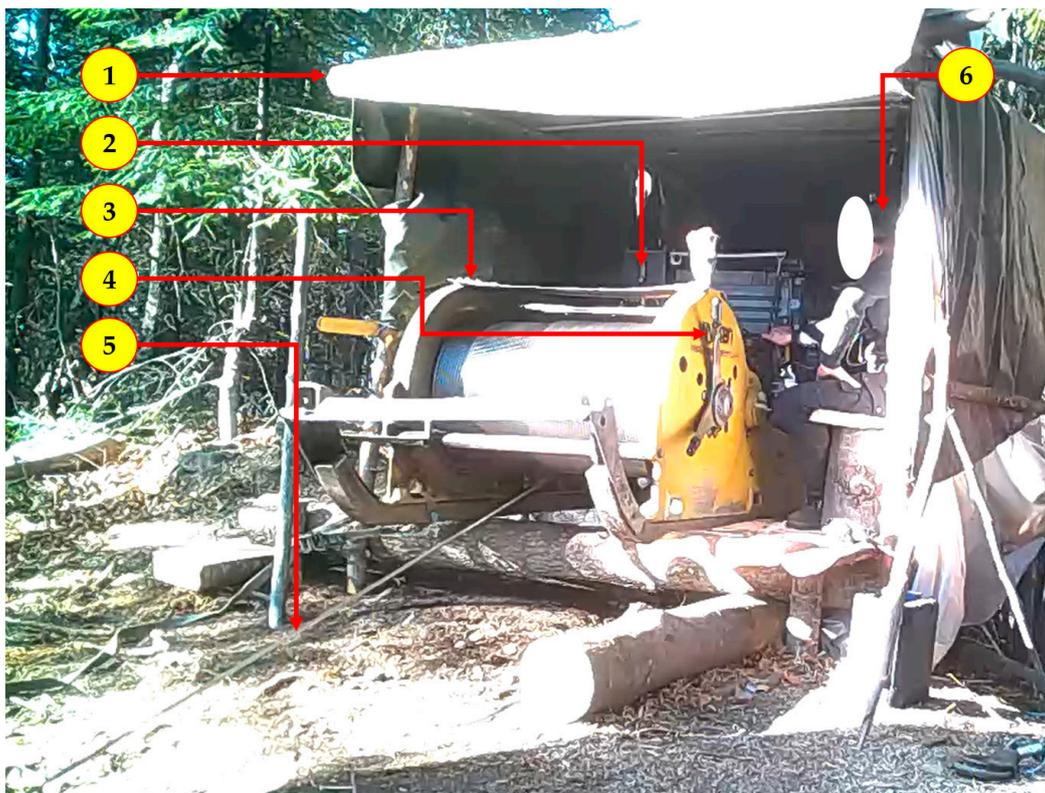
**Figure 2.** Description of machine under study: 1—machine protection against adverse weather built on site, 2—location of air brake, 3—drum of mainline, 4—lever controls, 5—mainline, 6—placement of noise dosimeter on worker’s helmet.
