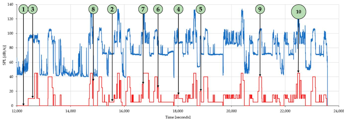
**Figure 1.** Example of event-based distribution in the time domain. Note: continuous blue line stands for instant readings of the sound pressure level (SPL) measured in dB(A); continuous red line stands for the occurrence of events described in Table 1: 1—engine off, 2—engine off, cooling, 3—engine on, no work, 4—cable work, 5—lifting the cable, 6—lowering the cable, 7—lifting the load, 8—lowering the load, 9—empty turn, 10—loaded turn.
