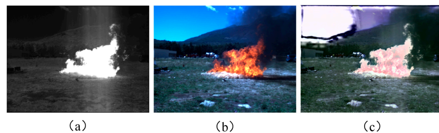
Figure 7. Test results of VTW-GAN after training on Corsican Fire dataset: (a) infrared image; (b) visible image; (c) fusion results.
