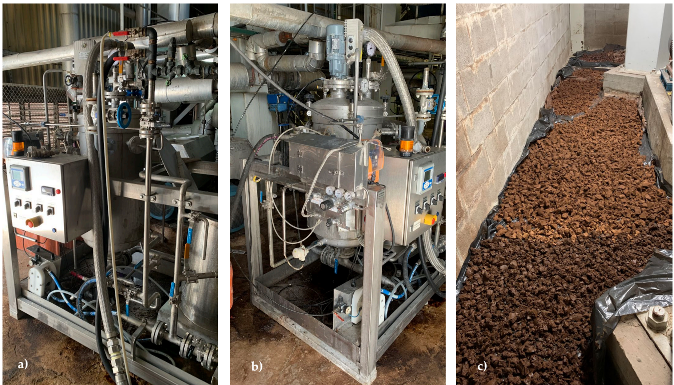
Figure 1. Images (a,b) representing pilot unit used for lignin precipitation and (c) shows the produced pilot lignin.
