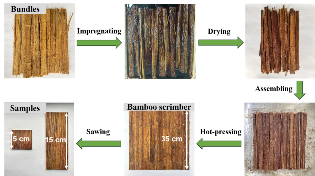
Figure 1. Detailed preparation process of bamboo scrimber.
