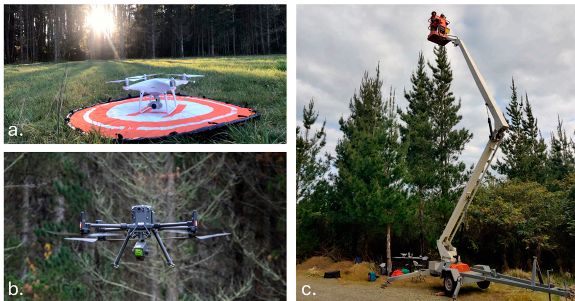
Figure 3. Images of the UAVs utilised in this study: (a) the DJI Phantom 4 Pro; (b) the DJI Matrice 300 RTK with a DJI L1 sensor. (c) Shows the flight crew operating UAVs from an MEWP to maintain VLOS.
