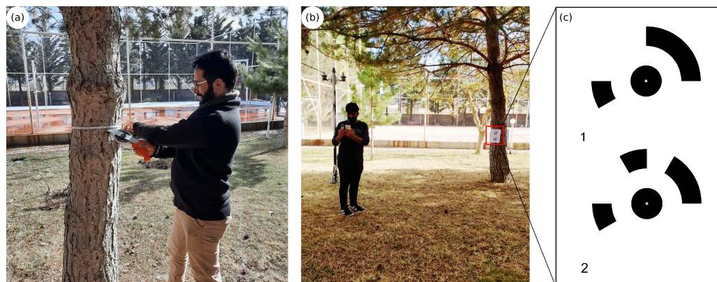
Figure 5. Field measurements: (a) tape measurement of the DBH, (b) image acquisition, and (c) RAD-coded targets with IDs.
