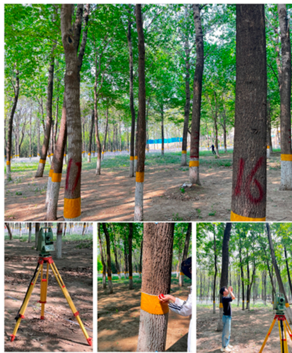
Figure 2. Actual data collection site. The photo shows the operator using a laser-based hypsometer to measure tree height at an approximate distance of 12 m from the target tree. During field measurements, a consistent distance of 10–15 m was maintained to ensure canopy visibility and the accurate detection of tree tops. The laser hypsometer provides strong canopy penetration ability and ensures reliable tree height estimation in open park environments.
