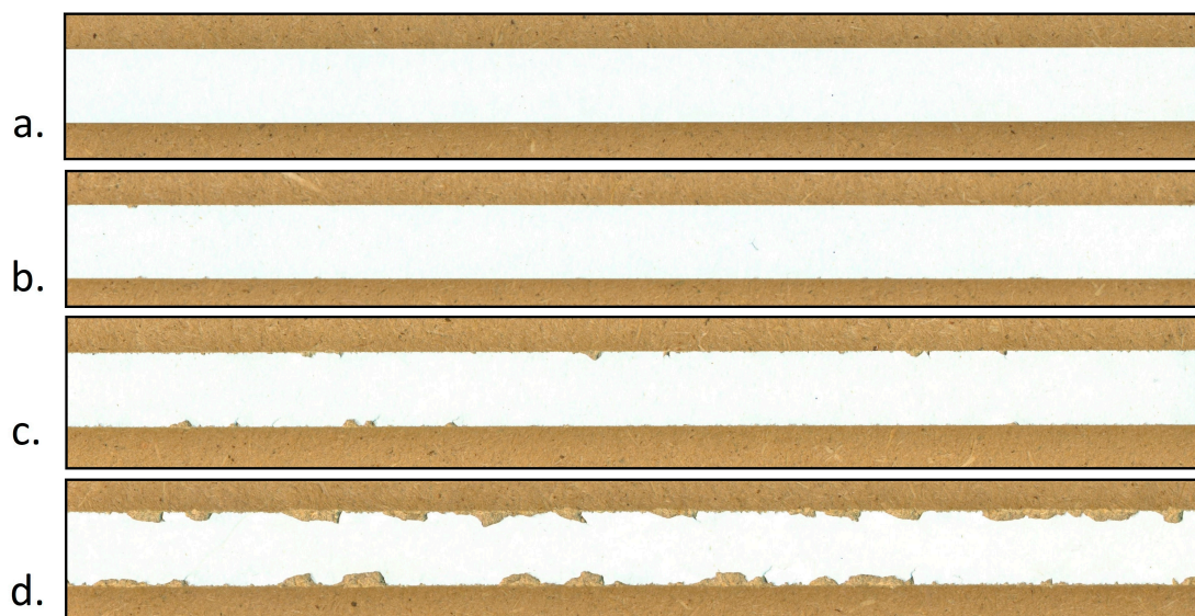
Figure 4. Example images representing different classes: (a) Class I (VB = 0–0.1 mm); (b) Class II (VB = 0.1–0.2 mm); (c) Class III (VB = 0.2–0.3 mm); (d) Class IV (VB = 0.3–0.4 mm).
